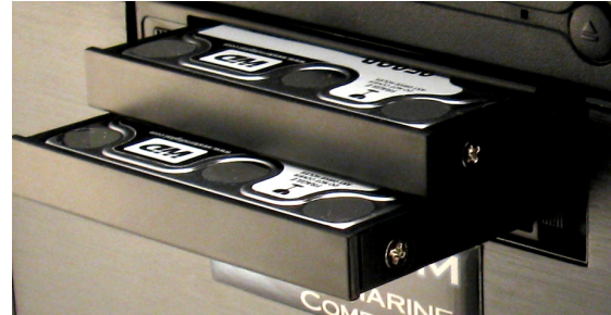
R.A.I.D. Module With Front Accessible Hard Drives
